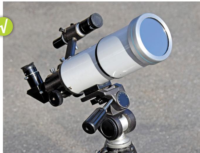
When using a telescope to observe the Sun at any time other than during the total phase of the eclipse, you must put a safe solar filter over the aperture (front) of the telescope, as shown here. Note that the small finderscope has been capped; this prevents concentrated sunlight from melting the crosshairs in its eyepiece.
